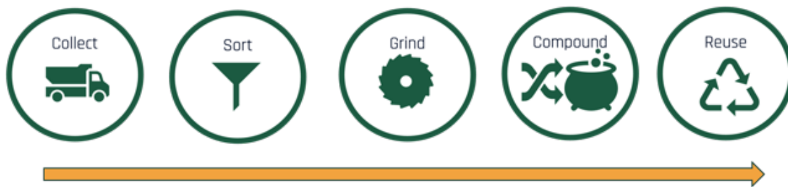
Figure 1. SPIRAL's solution of open loop recycling of TPC waste
